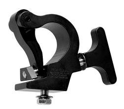
The new standard for hanging intelligent lighting fixtures. Allows one man to hang intelligent fixtures. Simply flip the link up, place clamp over the pipe and the Mega-Claw holds the weight of the fixture for you while you secure it with the solid 3/4" thick handle. The Mega-Claw will fit onto (I-I/2" Pipe) I.9" OD to 2" OD.
